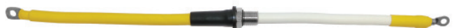
FT-SIL-80 HV Feedthru, single wire, silicone, max. 80 kVDC (not for silicone oil)
